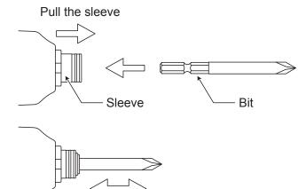
Release the sleeve and make sure the bit does not come off
