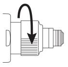
**3** Remove the spring plate assembly
