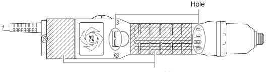
Fixing position of fixing jig
