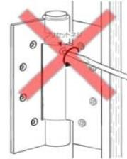
Do not loosen the preset screw before driving the spring pin.
