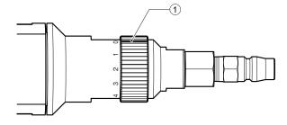
2 Turn the Valve Ring counterclockwise (②) until its red line (①) comes to the carved seal position "4"
