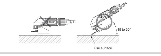
This tool is a pneumatic hand-held sander for polishing/grinding steel materials, etc. using the Abrasive Disc.
