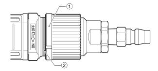
2 Attach the Connecting Hose to the tool, then turn the Valve Ring counterclockwise (4) while pushing the Valve Ring in the direction of 3
